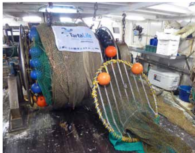
The Flexgrid during fishing operations and detail of a rigid TED used in sea trials.
